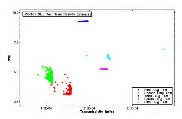
Figure 14. Formation transmissivity comparison from IMC-461 slug tests.
