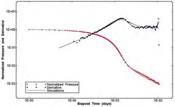
Figure 20. Log-log Ramey B plot showing 96 simulations of the IMC-461 response for slug test 3.
