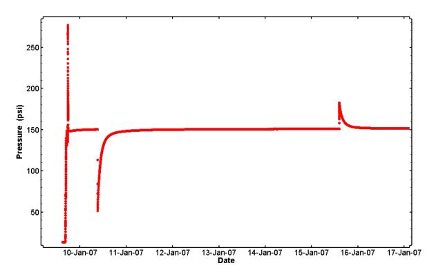
Figure 26. Pressure data from slug tests of the Magenta in C-2737.
