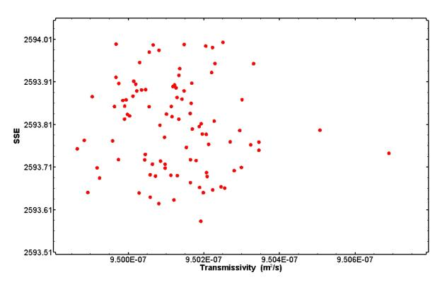
Figure 45. XY-scatter plot showing 96 estimates of transmissivity derived from the H-15 perturbation analysis.
