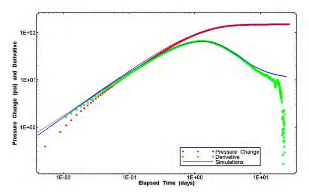
Figure 40. Log-log plot showing 97 simulations of pressure change and derivative during the H-11b2 pressure-buildup test.
