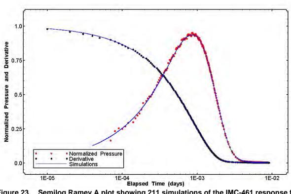
Figure 23. Semilog Ramey A plot showing 211 simulations of the IMC-461 response for slug test 5.
