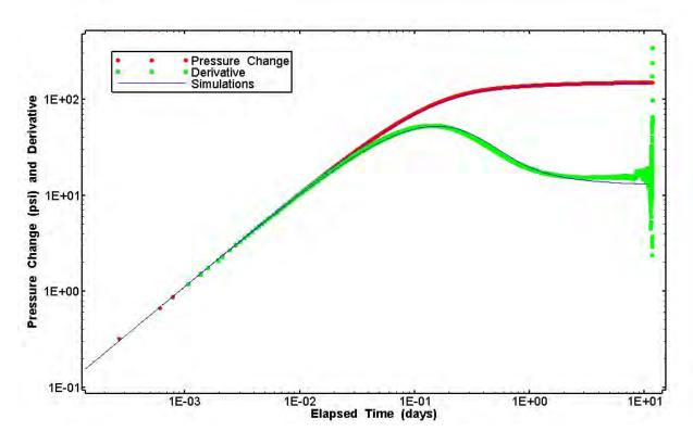
Figure 48. Log-log plot showing 96 simulations of pressure change and derivative during the H-15 pressure-buildup test.
