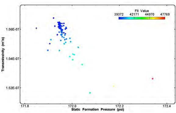
Figure B-8. Estimates of formation transmissivity and static formation pressure derived from the H-11b2 perturbation analysis.
