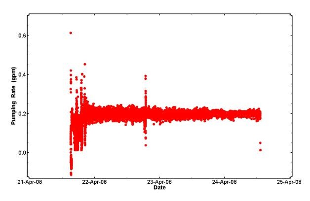
Figure 37. Flow-rate data from the Magenta pumping test in H-11b2.
