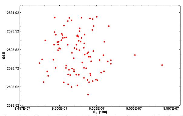
Figure B-11. XY-scatter plot showing 96 estimates of specific storage derived from the H-15 perturbation analysis.
