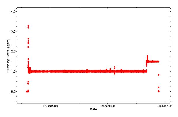
Figure 43. Flow-rate data from the Magenta pumping test in H-15.
