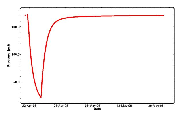
Figure 36. Pressure data from the Magenta pumping test in H-11b2.
