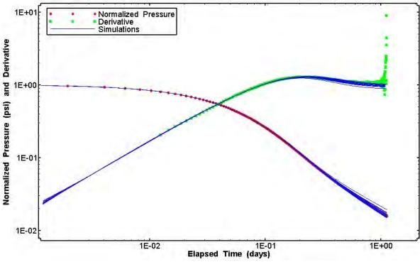
Figure 30. Log-log plot showing 43 simulations of the C-2737 slug-withdrawal test Ramey B and derivative response.
