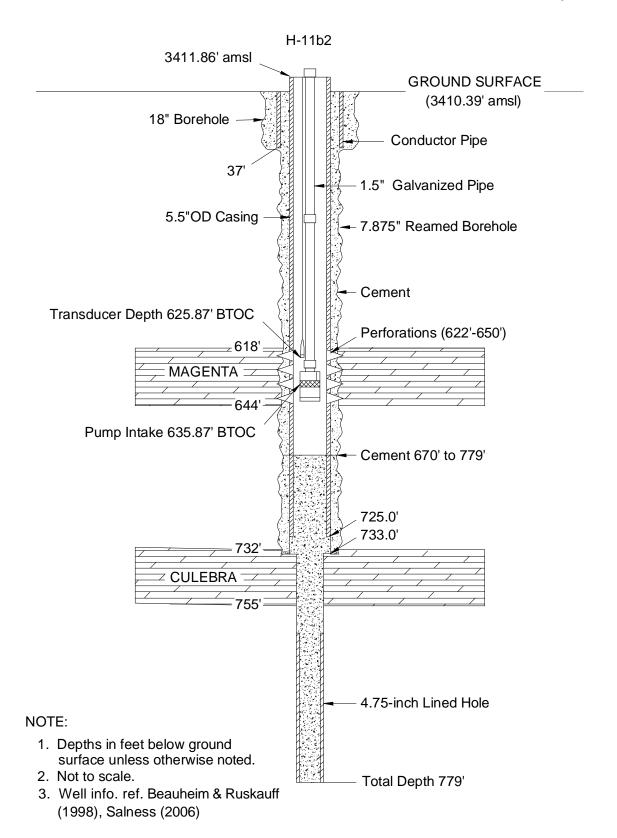
Figure 35. Configuration of well H-11b2 during testing.
