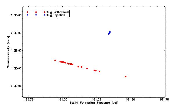
Figure B-4. Estimates of formation transmissivity and static formation pressure derived from the C-2737 perturbation analysis.
