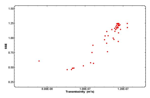
Figure 27. XY-scatter plot showing 43 estimates of transmissivity derived from the C-2737 slug-withdrawal test perturbation analysis.
