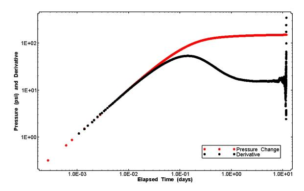
Figure 44. Log-log diagnostic plot of the H-15 pressure-buildup test.
