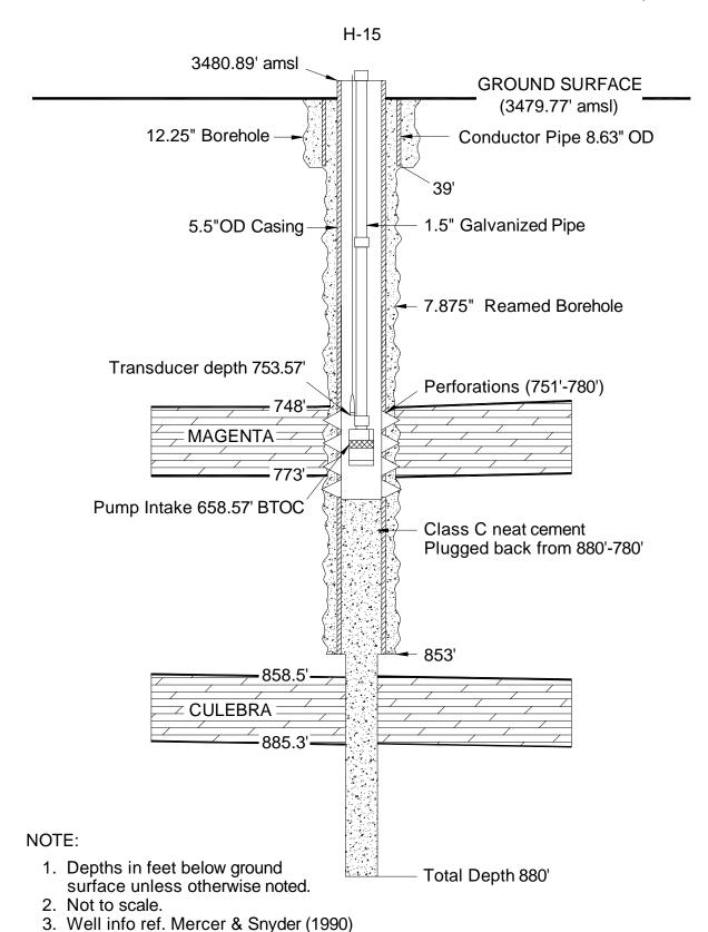
Figure 41. Configuration of well H-15 during testing.
