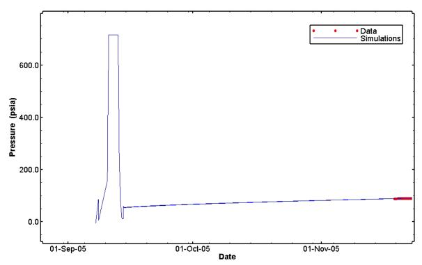
Figure 8. Simulated pressure-history for SNL-6 from well completion records.
