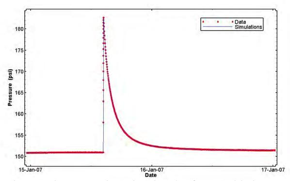
Figure 32. Linear plot showing 59 simulations of the C-2737 slug-injection test response.
