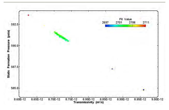
Figure B-1. Estimates of static formation pressure and transmissivity derived from the SNL-6 perturbation analysis.
