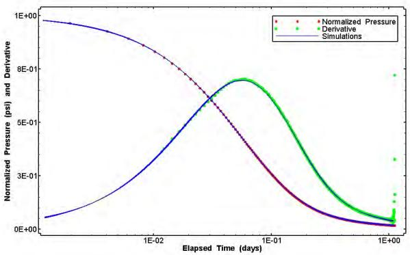
Figure 29. Semilog plot showing 43 simulations of the C-2737 slug-withdrawal test Ramey A and derivative response.
