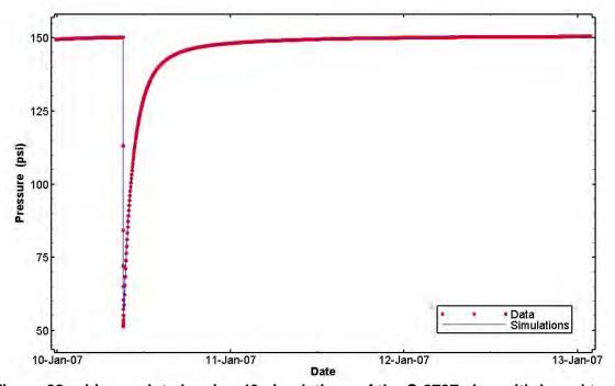
Figure 28. Linear plot showing 43 simulations of the C-2737 slug-withdrawal test.
