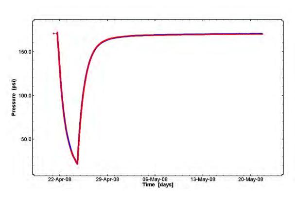
Figure 39. Linear plot showing 97 simulations of the H-11b2 pressure response.
