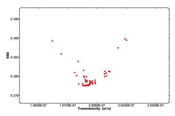
Figure 31. XY-scatter plot showing 59 estimates of transmissivity derived from the C-2737 slug-injection test perturbation analysis.
