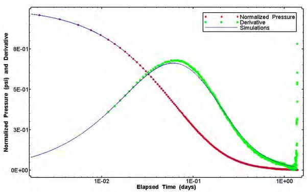
Figure 33. Log-log plot showing 59 simulations of the C-2737 slug-injection test Ramey A and derivative response.
