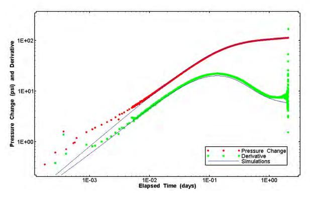
Figure 47. Log-log plot showing 96 simulations of pressure change and derivative during the H-15 pressure-drawdown test.
